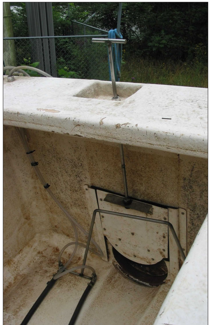
Figure 4. Slide gate located on the inside of a fiberglass tank.
